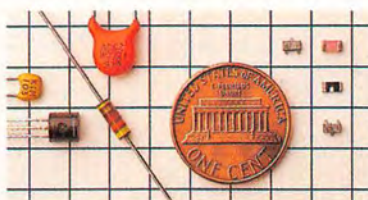
In PASSPORT, 102 SMDs (right) do the work of ordinary transistors, resistors and capacitors.
