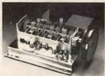
A five gang variable capacitor for FM reception that never varies.
