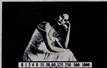
The match-needle viewfinder: just align two indicators for correct exposure. Because you're doing some of the work, you can save some money.
