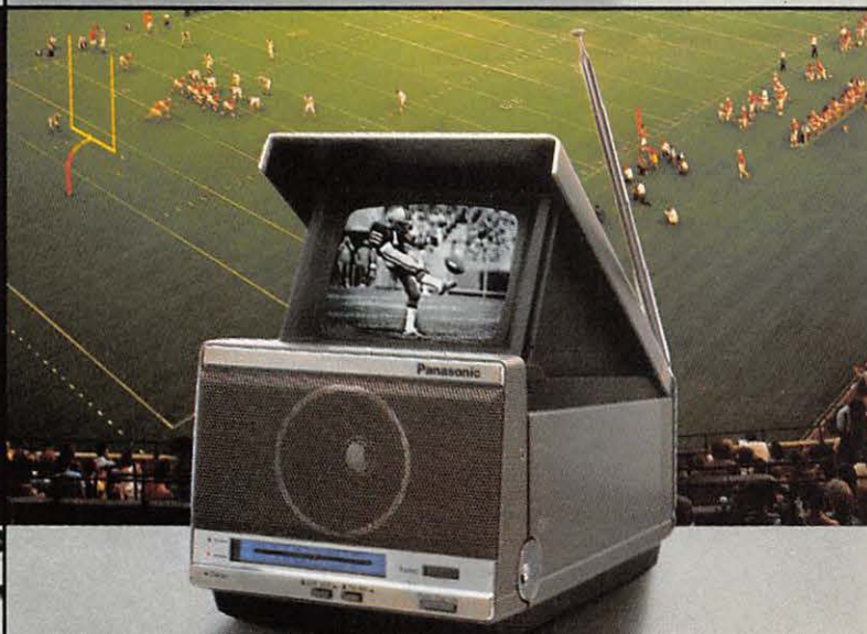
TR-5100P Portable. 5" TV that pops out of an AM/FM radio. Glare guard for better outdoor viewing. Plays on house current. Rechargeable batteries. And car battery with optional cord.
